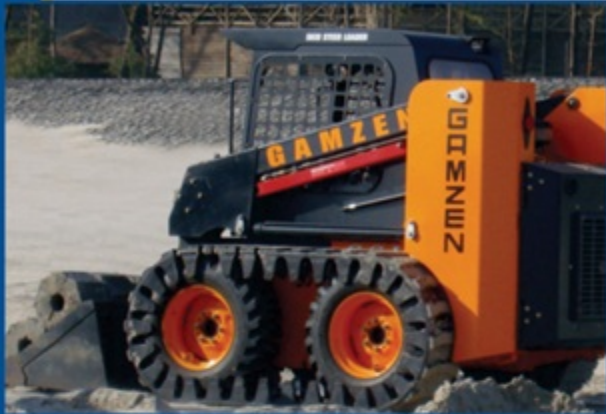
Skid Steer with Rubber Track for Sand and Marshy Land Work
